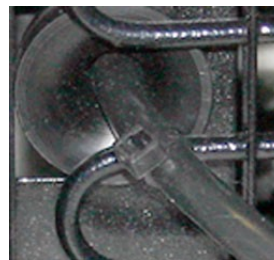
Figure 15: Cut cable tie to free line cord
