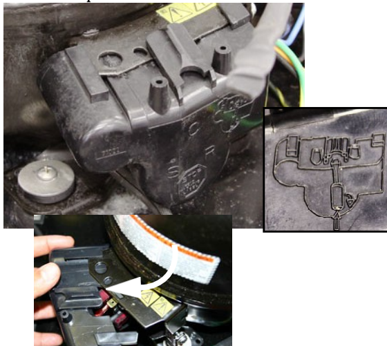
Figure 4: Access compressor overload A screwdriver may be used to release the latch.
